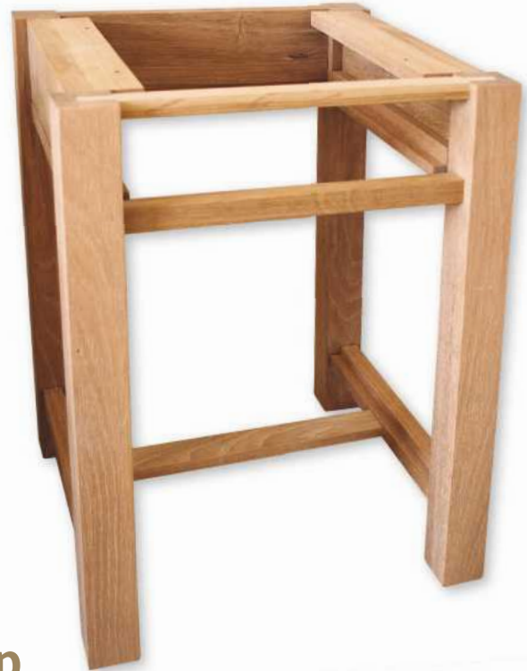
▲ Pic.4 The lower rails are rebated to receive the 8mm plate glass shelf
